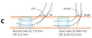
Tracheal defects caused by a commonly used round tube and the OctaTrach Oval tube
